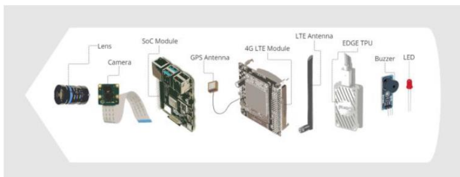
Figure 3: Device hardware components.
