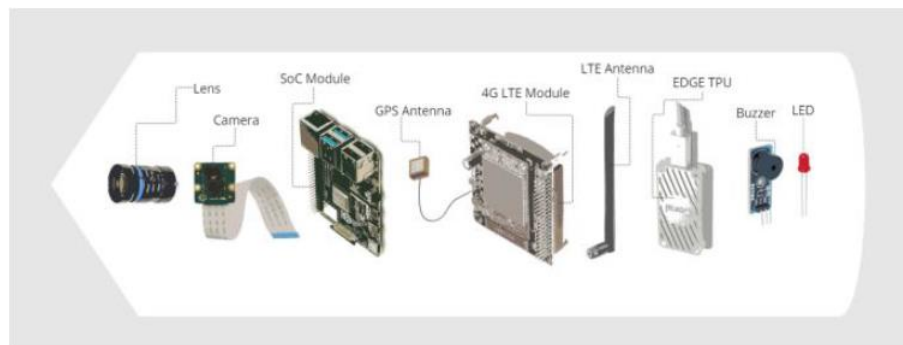
Figure 3: Device hardware components.
